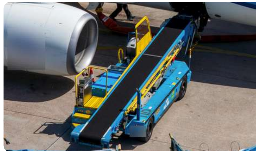
46.6 kWh Baggage belt loader
